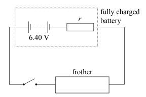
At maximum speed the power output of the frother is 4.5 W and this is achieved when the voltage across it is 6.25 V.
