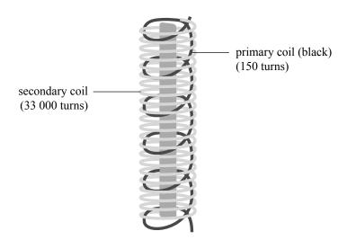
Current from the battery flows through the primary coil. When the circuit is suddenly broken, the magnetic field in the primary coil, and hence also in the secondary coil, collapses (falls rapidly). The mutual induction that takes place between the two coils produces the high voltage needed to create a spark.
